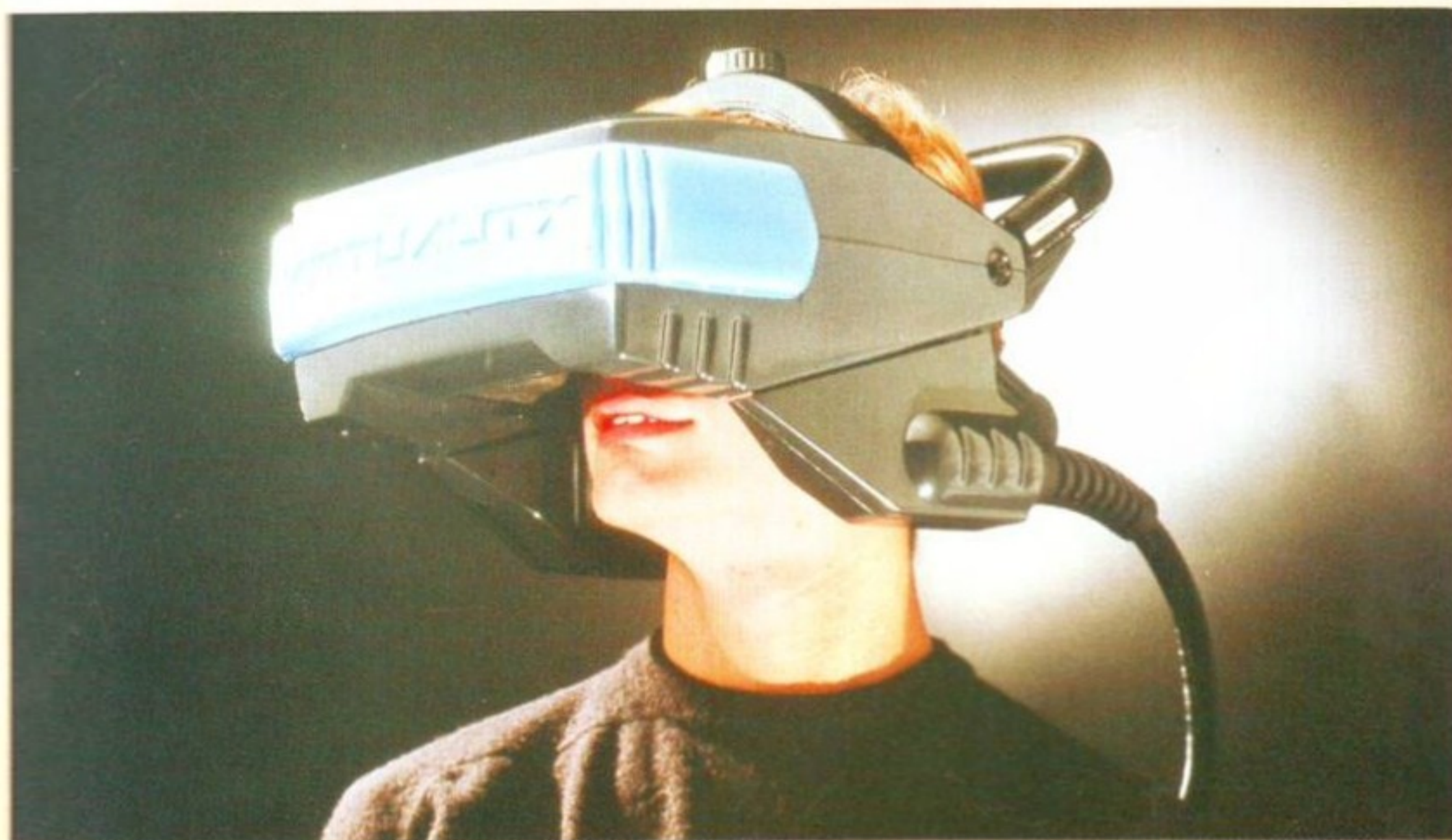
The helmet, or Visette, which is the main interface between operator and the virtual world.
