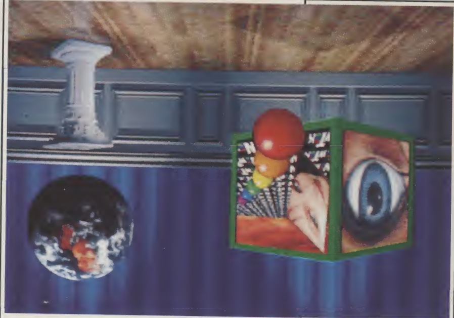
(below) This image demonstrates the use of Texture Mapping (the cube and perspective floor), user controllable Transparency (the reflections on the floor and the wall) and the 4096 color Hold and Modify mode.
