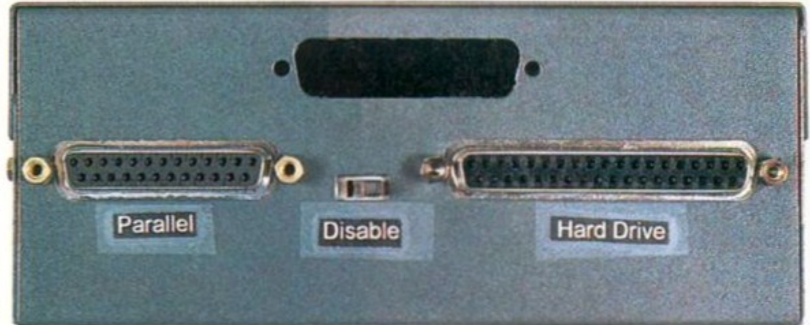
The hard drive connector can be used to add an external IDE mechanism. These are a lot cheaper than SCSI mechanisms.
