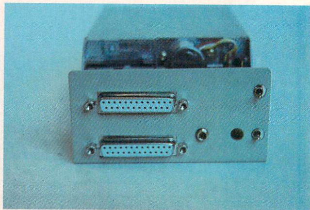
Left: Twindrive next to the Amiga 1010 disk drive. The former's super slimline packaging allows the user to conserve desktop space. Right: Twindrive's rear panel, showing pass-thru connectors and drive enable/disable toggle switches.
