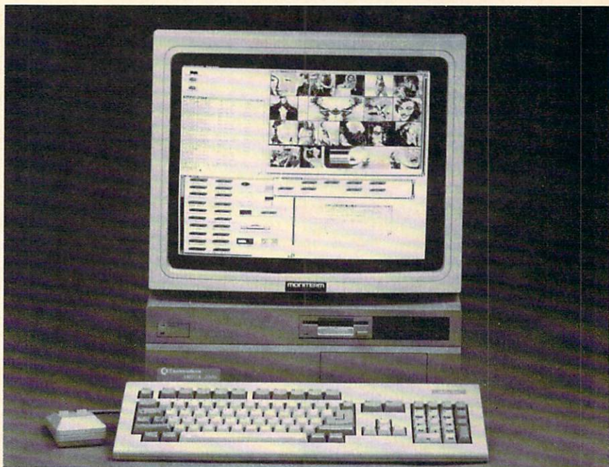
The Viking 1 is designed to expand the Amiga's capabilities for sophisticated applications in which a high resolution, non-interlaced monitor is preferable.
