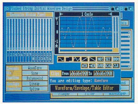
Above: the Plucked String design screen is typical of all of Synthia's working screens. Right: an iconic conceptual representation of Synthia's five instrument creation modules. READER SERVICE NO. 107
