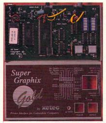
Inside Super Graphix Gold lurks (left to right) 32K of ROM, 32K of RAM, and an 8 bit 6303 microprocessor. The 5V regulator is at upper left. Switch settings are clearly labeled on the cover. READER SERVICE NO. 255
