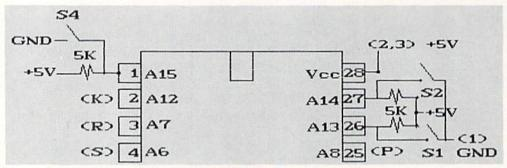
Figure 6: Modification for Bank Switching a 27512 EPROM
