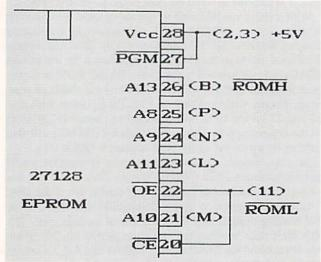
Figure 3: Modification for 27128 in \$8000 to \$BFFF Block
