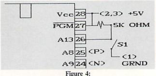
Modification for Bank Switching a 27128 EPROM S1 Open = Top 8KS1 Closed = Bottom 8K
