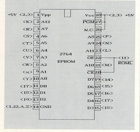
Figure 1: Connection to C-64 Cartridge Port
