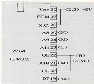
Figure 2: Modification for Cartridge in \$A000 Block
