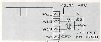
Figure 5: Modification for Bank Switching a 27256 EPROM
