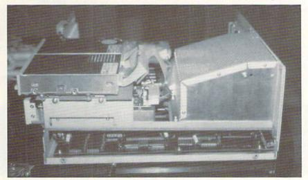
View from right shows disk drive stack and power supply enclosure. At bottom we have tantalizing glimpses of the RAM, ROM, and microprocessors.
