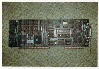
The Janus or Bridge board (actual name not yet set) is a ½M IBM PC clone on a plug-in card. Zorro connector is to the left with PC connector to the right.
