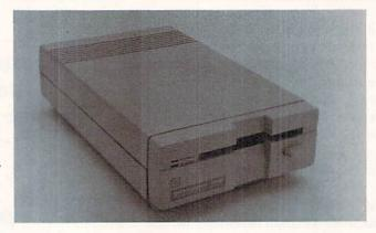
The Commodore 1581 3.5" disk drive has a data transfer rate three times that of the 1541, and over 800K storage capacity per disk. READER SERVICE NO. 158
