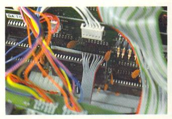
Installation of 21 Second Backup in an SX-64. Access to the VIA chip is more difficult than on the 1541 (below). READER SERVICE NO. 280
