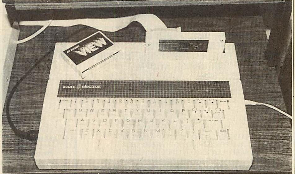
The Electron and Plus-1 combined with the AP-4 make a basic system for schools
