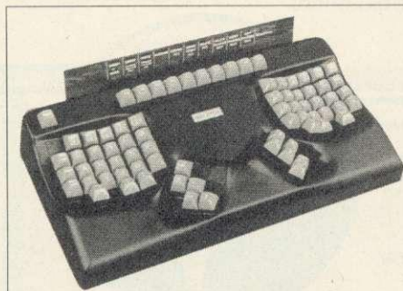
The unconventional layout of the Maltron
