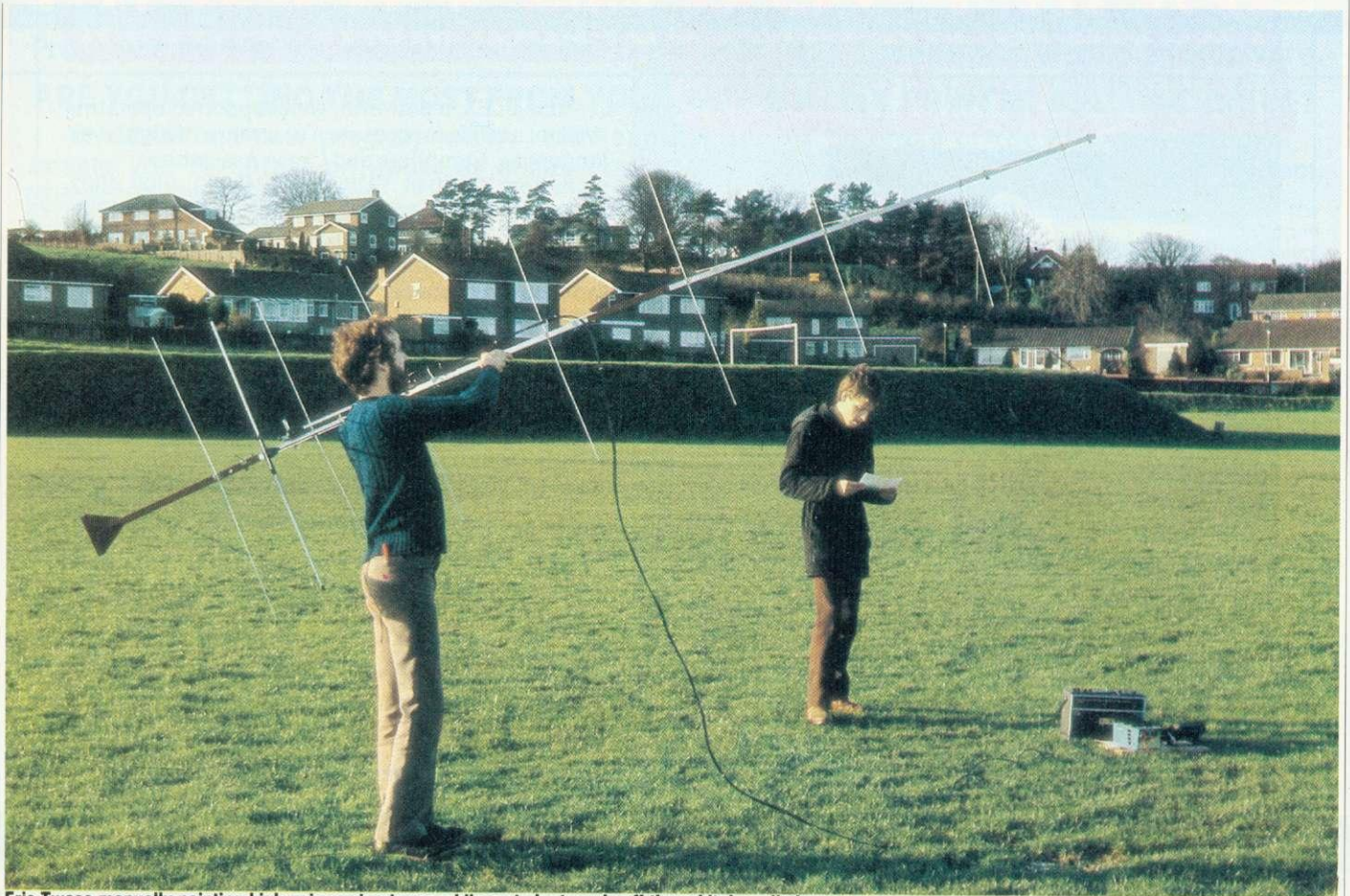
Eric Twose manually pointing high gain yagi antenna while a student reads off the orbital prediction
