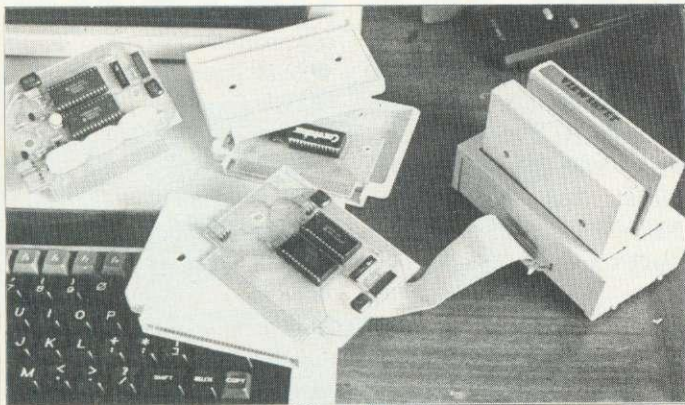
Voltmace battery back-up with 16k of RAM fitted (left); Caretaker ROM in cartridge; 4k ROM in uncased cartridge; buffer box with two assembled cartridges in place.
