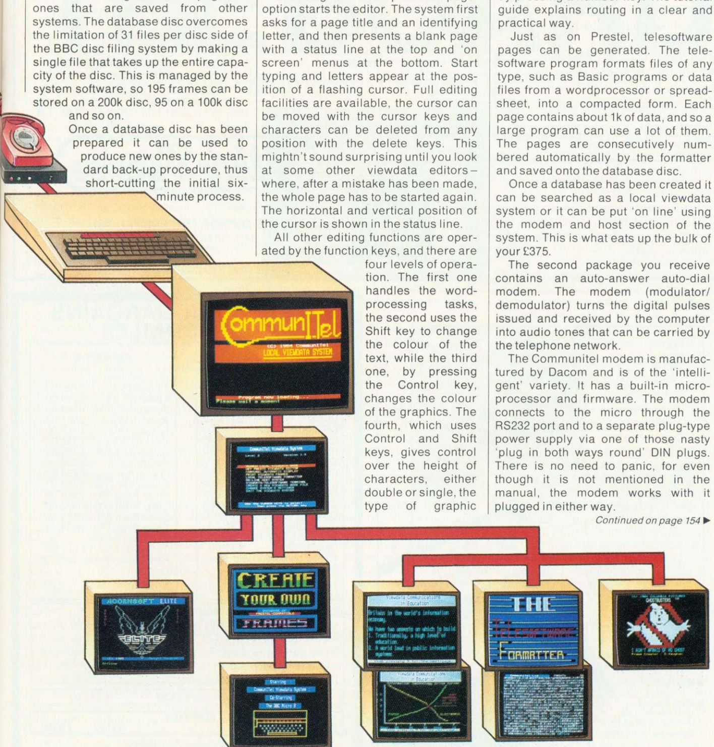
The Communitel system creates a Prestel-type database with a 'tree' structure of connecting frames. Our picture shows how BBC micros can contact a 'host system' over telephone lines and access frames on the main database. The opening page leads to sub-menus which in turn lead into display pages. Only the system operator can access the editing frames. Computer programs can be transferred to users by telesoftware
