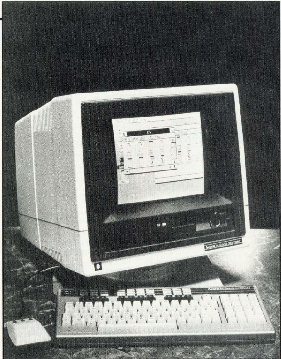
A marvel on marble: the ABC310 in all its glory. Beneath the monitor screen on the left is the Winchester hard disc, with the floppy drive beside it. Note the new symbols on the keyboard, re-arranged function keys, keypad and the mouse. There is no break key, but a reset is fitted on the rear of the keyboard. The monitor can be tilted and swivelled on its stand
