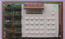
Micro" at this point you're sadly mistaken the first ever Acorn computer was the System 1. Sporting a 1MHz 6502 processor, 1K of RAM, hexadecimal output, and a rather bizarre keyboard, the system 1 could be yours in kit form for a mere £70.20 (in 1979 of course!)
