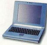
Magnesium Alloy Casing, Weighs Only 1.3Kg !, As small as 242 x 190 x 30mm!, 8.4" TFT 800x600 Colour Screen, 64Mb RAM Onboard., 10Gb IDE HD, Touchscreen, GlidePoint Touchpad, PCMCIA Onboard, USB Onboard, 10baseT Ethernet Onboard, VGA Output with DDC support, Audio Input, Audio Output, Onboard Stereo Speakers, 20W 3 cell LiFe battery, RISCOS4 and Utilities.
