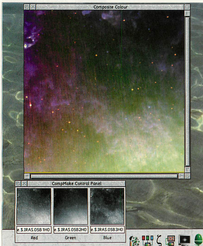
A colour composite image of a 12.5 degree square of the sky taken at three different infra-red wavelengths
