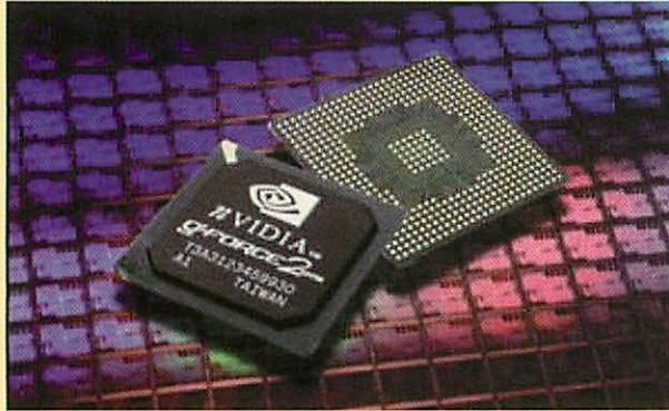
lighting removed from the computer's main processor onto the graphic card processor or GPU. The new card as well as adding the pixel-shading feature also sports improved 333MHz RAM and an Advanced Graphic port optimisation of x4 or 1024 MB/second. Initially the card is available in a 32MB version with plans for a 64MB version later this summer.
