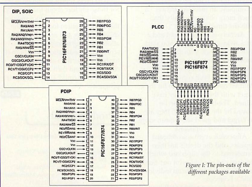
Figure 1: The pin-outs of the different packages available
