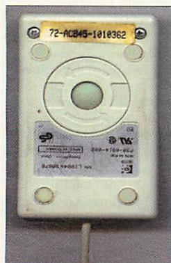
Figure II: Twist the circular section clockwise to release the ball
