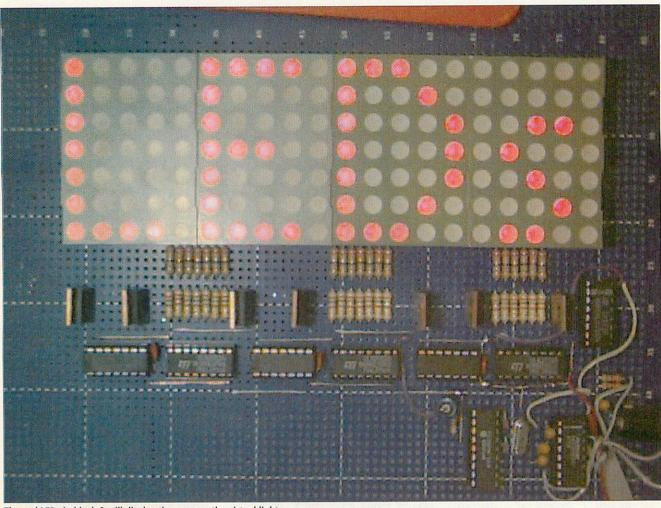
The real LEDs in block 0 will display the same as the virtual lights
