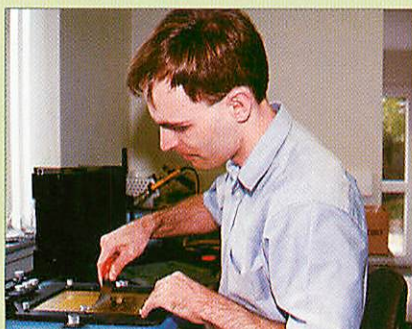
Spreading the solder across the stencil - where the stencil has holes, the solder paste will flow through onto the circuit board
