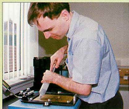
Applying the solder paste to the stencil for a set of A3000 memory upgrades
