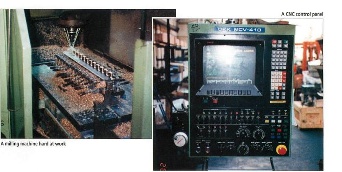
machines. This stores the programs and transmits them to the required machine on demand. Each program is stored as a number in its own dedicated directory for a particular machine. This is because usually each lathe or milling machine has particular strengths and weaknesses or subset of CNC commands. A program which would work on one machine might not necessarily work on another.
