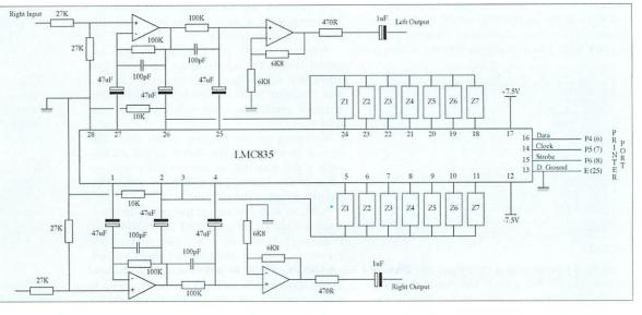
However, to get the maximum dynamic range out of the amplifiers these need to be powered with +/-15 volts.
