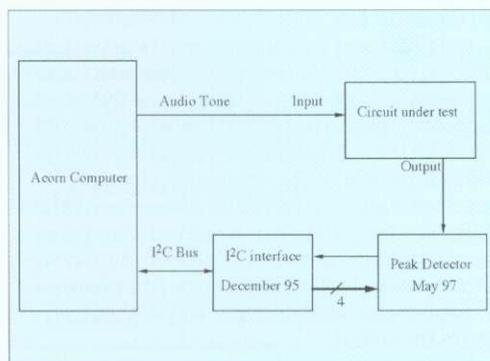
Figure I: The Frequency Response plotter set up
