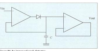
Figure IV: An improved peak detector
