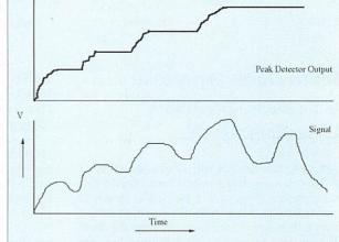
Figure III: The idealised output of a peak detector
