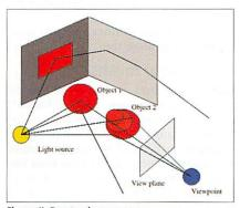
Figure II: Ray tracing a scene
