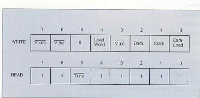
Figure I: FM Radio register structure
