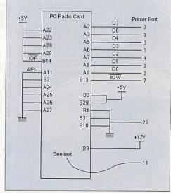
Figure II: Wiring up the board to the printer port
