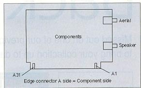
Figure III: The card's edge connector
