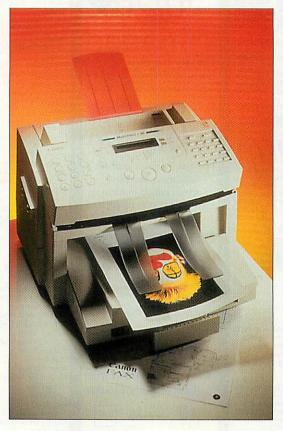
20-sheet document feeder for the 200dpi monochrome scanner section. At 200dpi, you will only get fax-resolution scans and copies, but it's better than nothing and scans take just six seconds per page. A telephone handset and an LCD status display are included. The MP10 will also work as a stand alone fax machine
