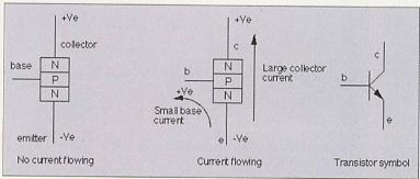
Figure I: A basic transistor
