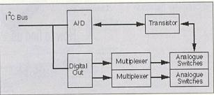
Figure IV: The block diagram of the transistor tester
