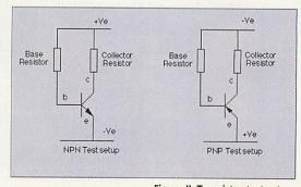
Figure II: Transistor test set up
