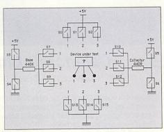
Figure III: Transistor tester switching arrangement
