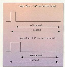
Figure 2: Decoded output
