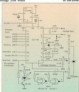
mV drop in the reading. However, if you can sacrifice the last digit you can go faster. A better, polypropylene capacitor will cost several pounds but should enable you to go at full speed.
