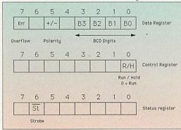
conversion was completed, the next one started. This time I am using that pin to command a conversion when one is needed, so all it needs is a quick blip to set it going.
