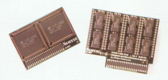
They will fit with all popular makes of existing 4Mb memory, ARM3 upgrades and podule expansion boards, providing the MEMC socket is not obscured. The 300, 400 series and 33Mhz A5000 computers just plug in with no soldering required. The A3000 and older (25Mhz) A5000 require a surface mount MEMC socket fitting to the motherboard. Please ask if you require this service.
