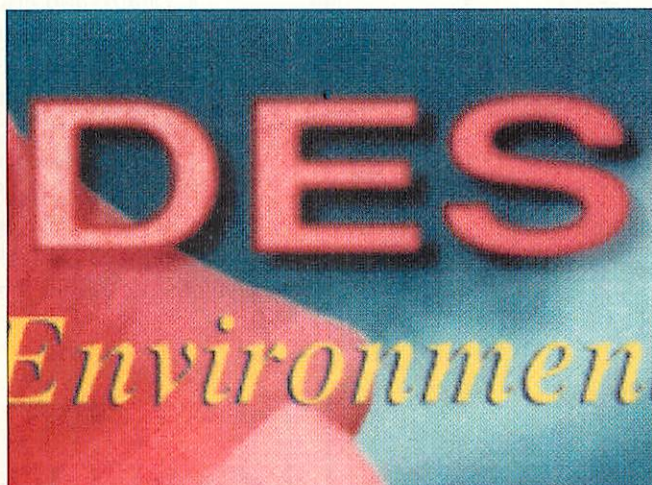
An 800dpi dye sublimation print (scaled up linearly by four), interpolated from 200dpi using Spacotech's error diffusion for unusually sharp dye sub text and line art.
