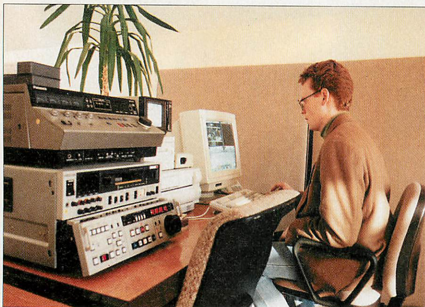
Mike Copperwhite of Eidos sitting in the Eidos 'video corner'. He is working at a Risc PC fitted with an ARM710 chip and an Apex digitiser, which will capture and compress 25 frames of VHS resolution video in real time. Envious? We are.
