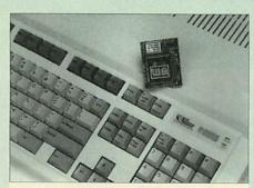
Using the latest surface mount technology on a high quality 4 layer circuit board we have reduced the overall size to a mere 53 x 45mm, and the cost to only £99. The ARM3 upgrade will increase the speed of your A300, A400 or A3000 computer by up to 6 times.
