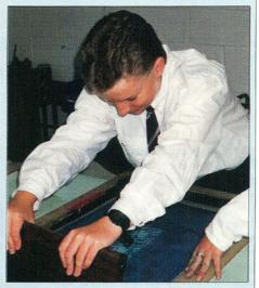
centre. Put a label underneath the cross, so it is printed on the label, not the fabric. All the unwanted areas of the screen must be covered using paper and tape. The darkest colour dye is put on the screen, above the area to be printed. A squeegee is then used to force the ink through the mesh and on to the fabric.
