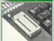
Allows you to change your ROMs quickly and efficiently, without having to open the lid. The ZIF socket is located into the ROM Cartridge's position. It is very simple to install. No soldering required. Also included in the price is a see-through storage case with antistatic lining, which allows you to store 12 ROMS. **£18**
