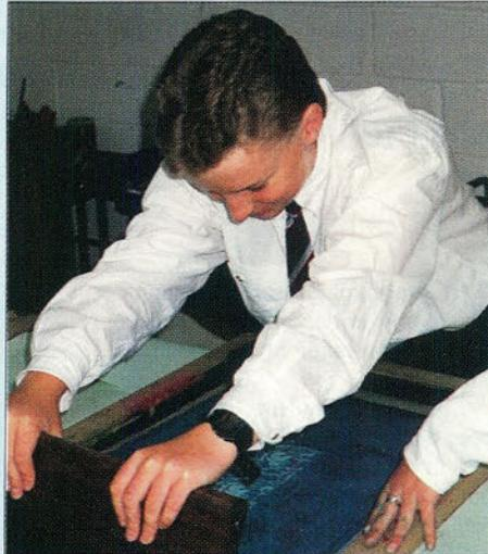
centre. Put a label underneath the cross, so it is printed on the label, not the fabric. All the unwanted areas of the screen must be covered using paper and tape. The darkest colour dye is put on the screen, above the area to be printed. A squeegee is then used to force the ink through the mesh and on to the fabric.
