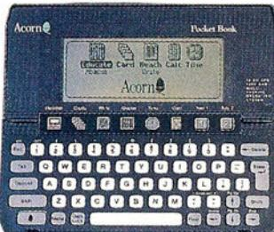
This enables database files to be entered and updated on an Archimedes using the *Desktop Office* database module and exported to the PocketBook/Series 3, or vice versa, through the Acorn A-Link serial port.
