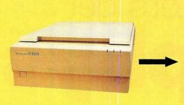
Scanning in illustrations is achieved using two flatbed scanners. The journal chose A4 flatbed scanners from DT Software, which can offer 1600 x 1600dpi maximum resolution and 24-bit colour scanning. Paint and Draw are used for image enhancement and Artworks for importing font-outlines and graphic files.
