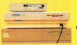
The Journal runs on A5000s with up to 8Mb Ram, and A540s with 12 or 16Mb Ram. They all have 120Mb hard drives and State Machine Graphics Cards and are linked into an Ethernet network with a 500Mb fileserver. The backups go onto a Syquest drive.
