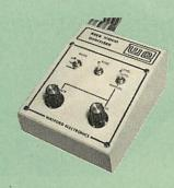
Using any source of composite video (colour or monochrome) and the Watford Beeb Video Digitiser, you can convert an image from your camera into a graphics screen on the BBC Micro.
