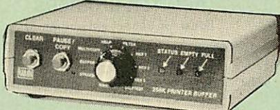
This new Megabuffer 256 from Watford is a full featured 256K Printer Buffer. It allows the computer to print 256,000 characters in a short time thus freeing the computer very quickly. In short it makes light work of printing large documents, screen dumps, etc. It is extremely simple to connect. The features are:
