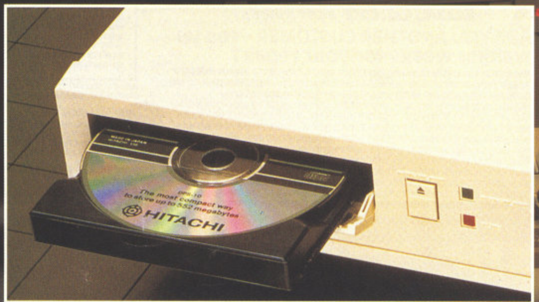
The Hitachi CDR 1503S – some £750 worth of advanced technology. The drive can be linked to a PC and used to load data from CD ROM, but it also doubles as an audio CD Player. Plug the drive into your HiFi as well as your PC and you can play Defender of the Crown with an orchestral soundtrack in full stereo – or switch the PC off and 'relax' to the latest Bon Jovi CD, if that is your musical taste...
