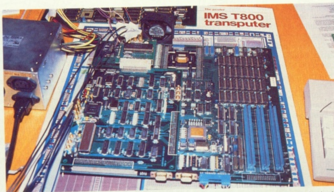
The multi-storey ABAQ motherboard: the three blue edge-connectors in the foreground take 'farm' cards or extra memory, while the micro-fan in the background keeps the whole thing cool!
