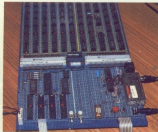
The SAM prototype. The nearer board is the computer itself, while the more cluttered one in the background handles the video logic: this'll be replaced by a single custom chip in the finished machine.
