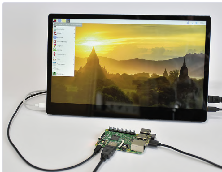
Figure 6: Here the Joy-View 13 is connected to a Raspberry Pi 3B running Raspbian.
