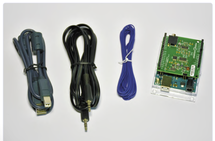
Figure 2: This you have to supply yourself: an Arduino Uno, USB cable, audio jack cable and a piece of wire.
