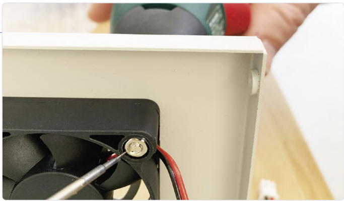
Figure 5: A fine-tipped screwdriver stops the nuts from spinning while tightening.
