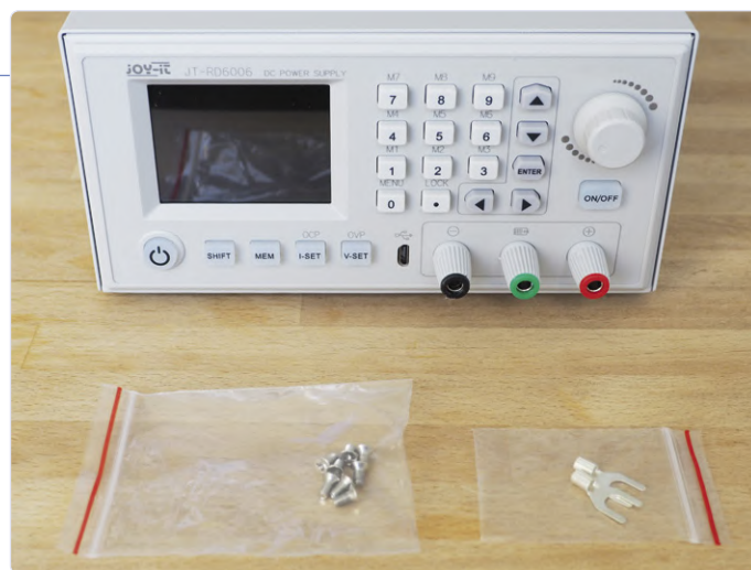
Figure 10: The finished benchtop power supply. I ended up with eight M3 countersunk screws and two cable lugs leftover.
