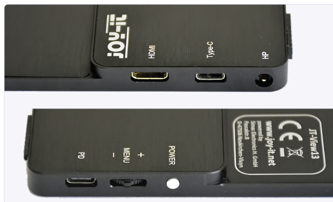
Figure 2: The connectors on the right side (top) and left side (bottom) of the Joy-View 13.
