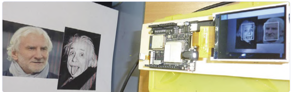
Figure 6: Test setup for face recognition.
