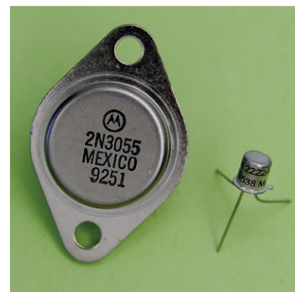
Photo 10: Comparing the size of two transistors. Tip: to avoid reflections from metal surfaces, you can grease them lightly.
