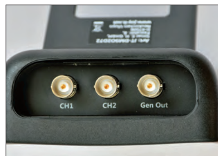
The BNC sockets are recessed quite low in the top of the cabinet.
