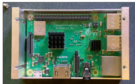
Figure 3. With an RPi 3 or 4, the lid needs to be left off if the board is built into an opaque or metal housing.
