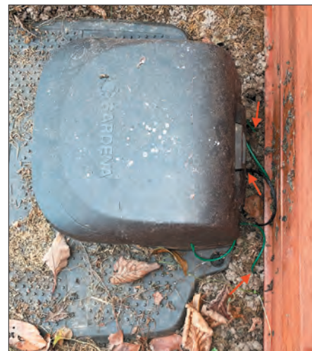
Figure 5. The charging point normally concealed in the kennel (here removed for inspection) with associated cables.
