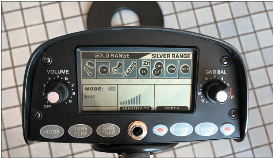
Figure 7. Display on a 'proper' metal detector. This is the CS-400 model by Velleman [1].
