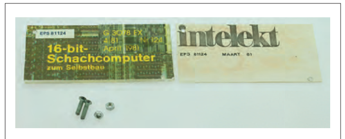
Figure 2: The Intelekt screw-on product descriptor plate set is reversible to show one of two languages: Dutch or German, depending on the show or demo location.
