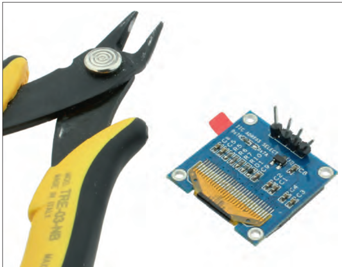
Figure 6. Use sharp cutters to snap into the plastic material between the pins until they are no longer held together.
