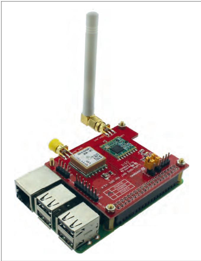
Figure 15. A Raspberry Pi with Dragino-LoRa-HAT acting as gateway.
