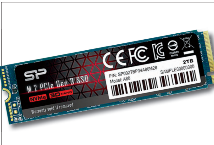
Figure 6: Fast M2-NVME-SSD ACE-A80 from Silicon Power (Image: Silicon Power [3]).
