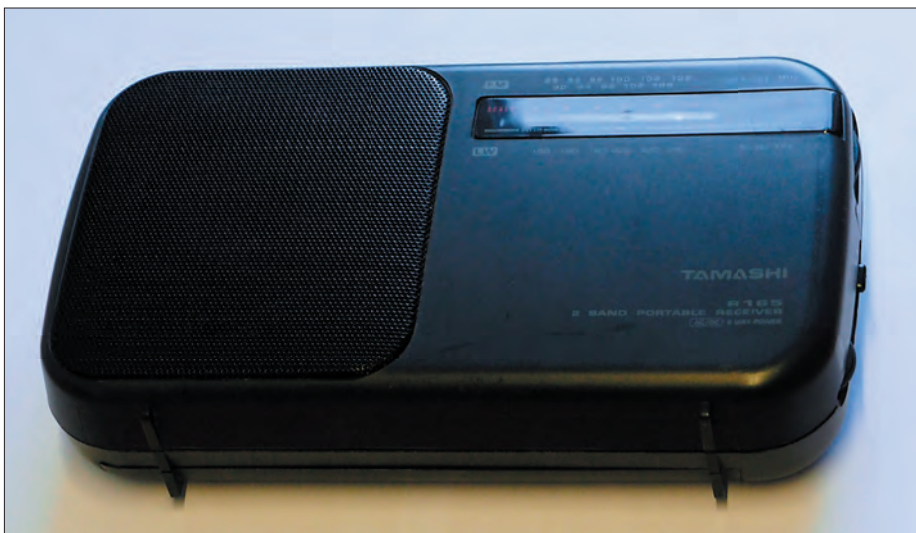
Figure 8. I bagged this basic portable radio with LW reception for a ridiculous amount on eBay. It serves as a universal receiver for detecting breaks in concealed wires.
