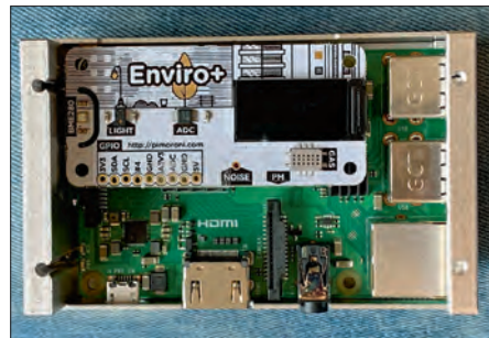
Figure 5. The Enviro+ with added tape on an RPi 3B+.
