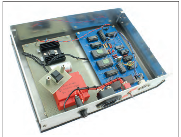
Figure 1: Intelekt case with the cover removed. The Interrupt pushbutton is a 'Digitast' type with tactile feedback!. Here it can be seen soldered on a small piece of perfboard with two standoffs, and connected to the circuit board with wires.
