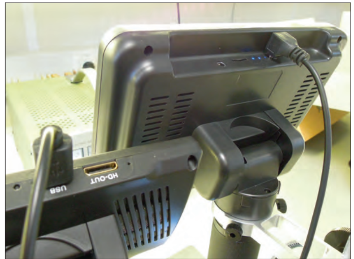
Figure 3. The cable will last longer thanks to the right-angle USB plug.
