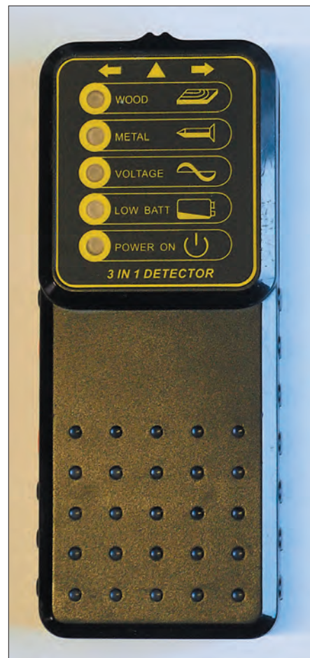
Figure 6. Simple metal detector, sold in DIY stores as a cable finder.
