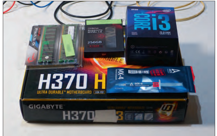
Figure 1: All the innards (motherboard, RAM, SSD, CPU and thermal paste) waiting to be assembled to make a lab PC.
