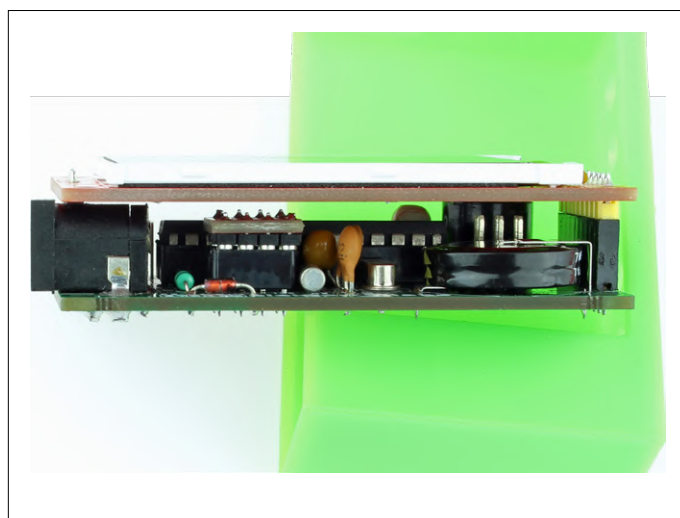
Figure 7. A sandwich made up of the clock PCB, BoB and display module with the SD card slot metalwork removed.
