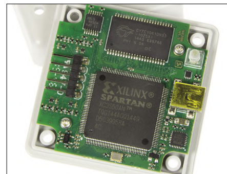
Figure 1. The innards of the ScanaQuad comprise mainly a Spartan FPGA made by Xilinx and fast memory.
