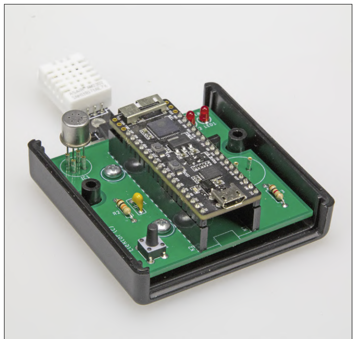
Figure 8: The prototype sensor unit fitted with the ESP32 and DHT22 Temperature sensor.
