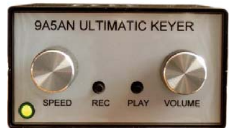
Figure 3. Suggested mounting in a metal case (author's prototype).
