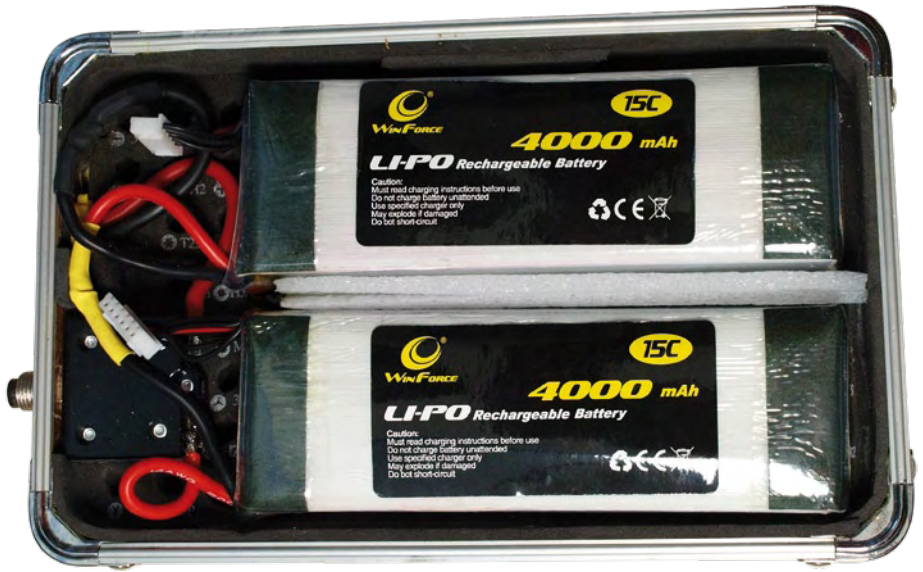
Figure 1. The power source for the author's electric bike. Two series-wired 5s LiPos from China built into a small aluminum case with a thermal fuse.
