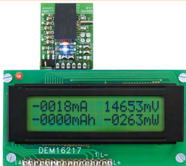
Figure 2. The connector used on Existing Elektor projects for connection of the USB to TTL cable from FTDI [1] will also plug into the Bluetooth-Dongle.
