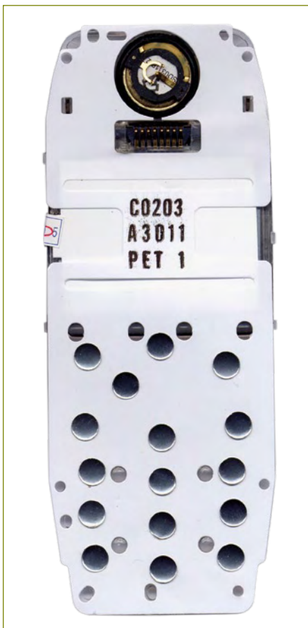
Figure 4. The display module consists of the actual display and a keypad section.
