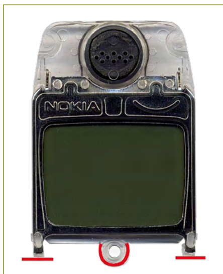
Figure 5. Saw through the plastic substrate along the red lines marked on this photo.
