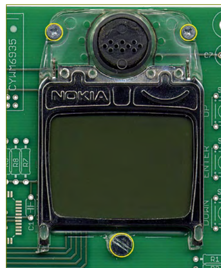
Figure 6. The display module is fitted to the PCB with two M2 screws and an M3 screw.
