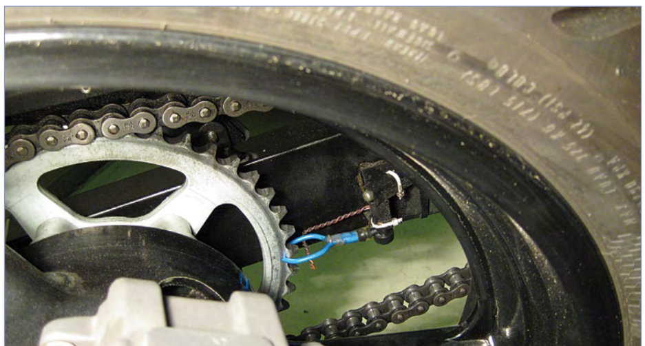
Figure 4. Rather than dripping oil on the chain and spilling most of it while riding, the dispenser lubricates the rim of the chain wheel.
