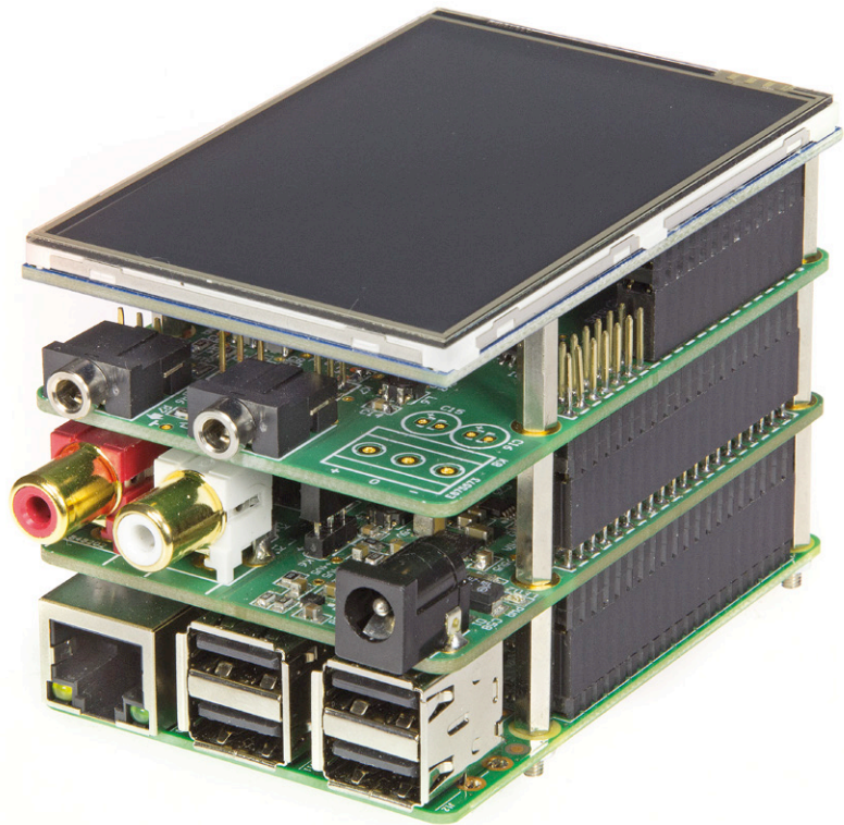
Figure 5. Here you can clearly see how the sandwich is put together.
