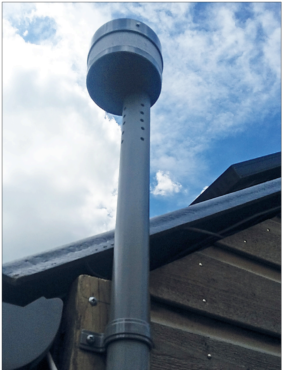
Figure 9. The wind gauge in its natural element, well above the roof.
