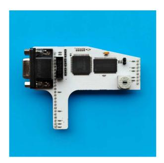
For most situations, you will simply connect the PCB to back side of your RamWorks card, and connect your VGA monitor to the VGA port.
