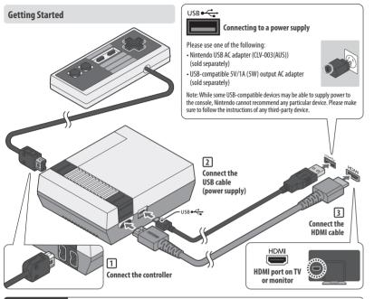
Make sure the connectors on the cables are oriented correctly and then insert them straight into the correct ports.
