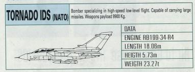
Standard bomber developed jointly by England, West Germany and Italy. Distinctive features are high-speed, low-level attack capabilities and deadly accuracy. It maintains its maneuverability during low-level flying and can follow the contours of the land at altitudes as low as 60 meters. Distinguished by accuracy at both high and low altitudes, and its sophisticated STOL capabilities. In addition, it is used by the English Air Force as an ambush bomber.
