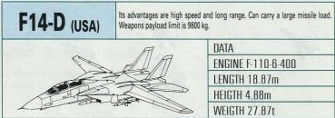
American Navy variable wing fighter. Usually assigned to squadrons in charge of air defense of aircraft carriers. It can track 24 targets simultaneously at long range, and attack 6 aircraft at the same time with its APG-71 radar and AIM-54C. Equipped with the latest Phoenix air-to-air missile weapons system.
