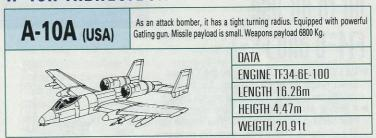
American Air Force bomber developed for the Vietnam War, it specializes in close support. With its heavy armaments it can remain over a battle zone long periods of time. It was developed for its maneuverability as well as its high survival rate in combat. Top speed of 722 km./hr. Unique appearance. Boasts a fixed large-bore 30mm Gatling Gun.
