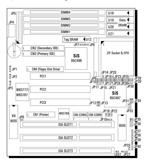
Figure 1. The main board layout
