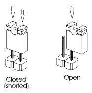
NOTE: When a jumper is open, keep the plastic cap inserted over one pin of the jumper so that you don't lose it.
