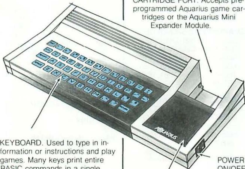
**KEYBOARD.** Used to type in information or instructions and play games. Many keys print entire BASIC commands in a single keystroke, when used with the CTL (Control) key.
